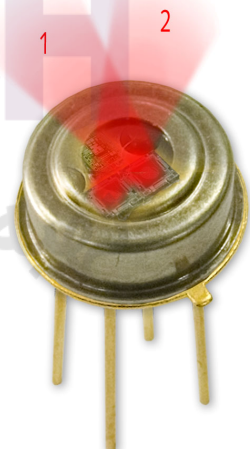
Figure 21: identification of zone 1&2 relative to alignment tab.
